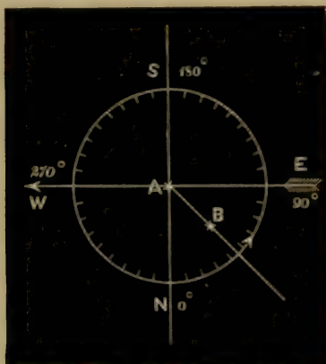
FIG. 38.—MEASUREMENT OF POSITION-ANGLE.
